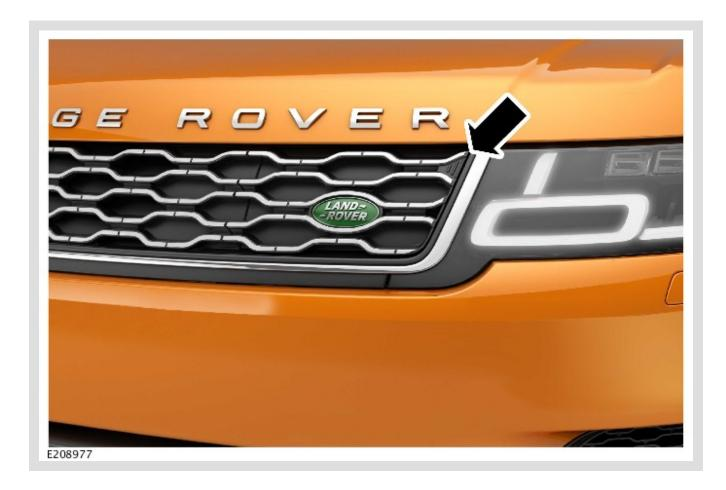
Behind the grill opening panel is the PHEV charge port.
