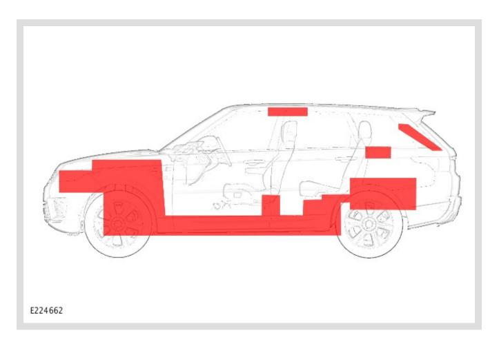
The sills must be supported during cutting and extrication procedures. If a ram must be deployed, place blocks under the sill around the area where force is applied. If a suitable jacking point cannot be located, support the sills and deflate the tires.
