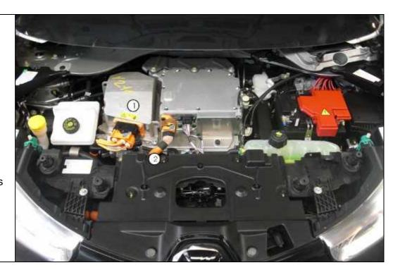
➤ The orange colour of the 400 V cables does not mean that these are "fire-resistant" cables.
